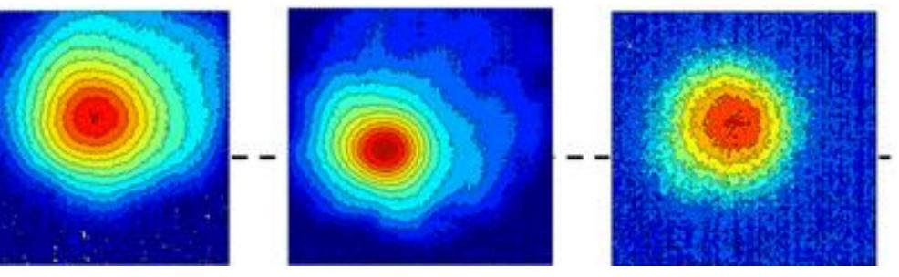
• Linking SLM melt pool data to microstructure data establishes a process-structure relationship that can become part of a more comprehensive digital material twin. • Image preprocessing steps before training the model: • Centering melt pool spot
