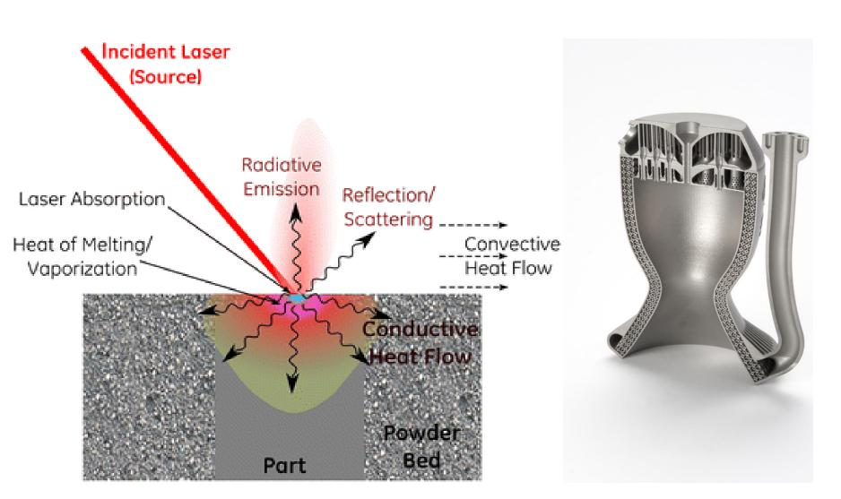
• Selective laser melting (SLM), is an AM process that involves using a laser to melt powder in a bed to produce metal components.
